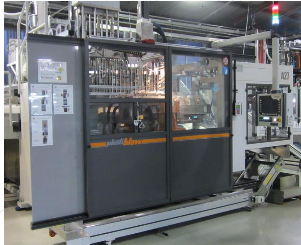
A new fully electric extrusion blow moulding machine (EBM) for the production of multi cavity bottles up to 5 litre size, reducing electricity consumption and creating a quieter, cleaner working environment. The machine's movements are fast and precise adding to the machine's efficiency and reliability
